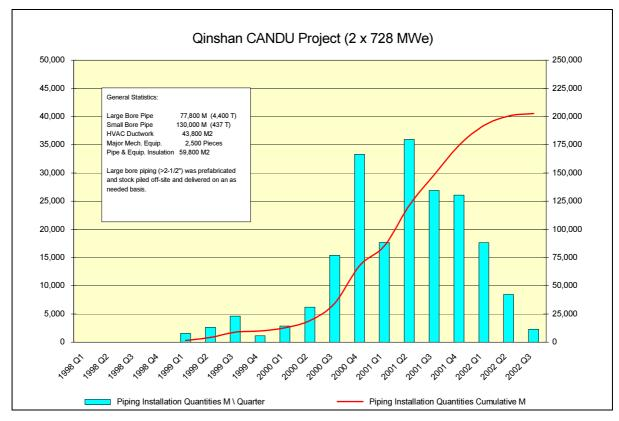
Fig. A.1.6. Mechanical works (Qinshan).
