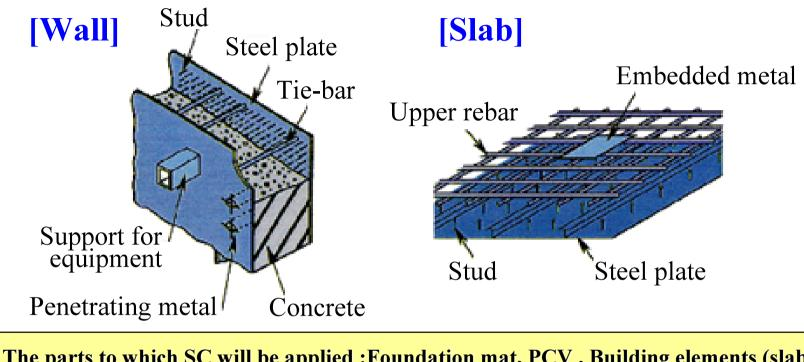
The parts to which SC will be applied :Foundation mat, PCV, Building elements (slabs and walls) - critical parts which affect the whole construction period )
