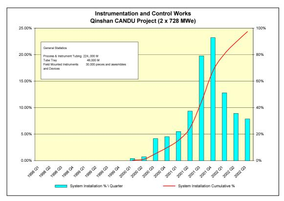
Fig. A.1.8. Instrumentation and control works (Qinshan).
